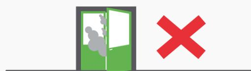
**Incorrectly controlled doors** can create a hole in your fire and smoke barrier
