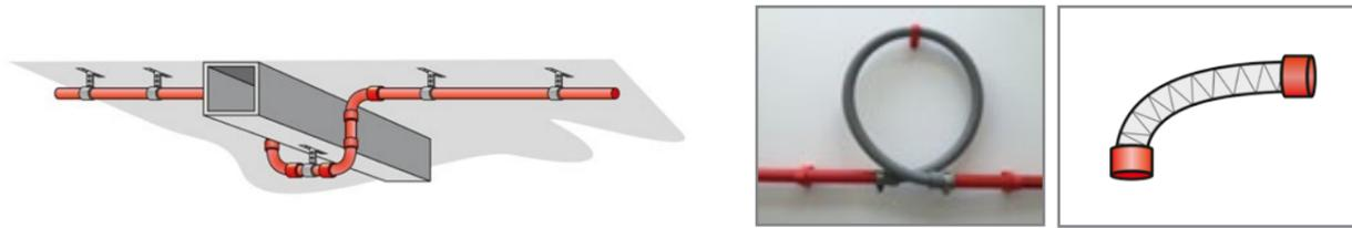
Figure 2. Expansion clip Flexible connector
